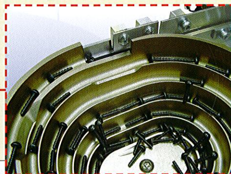
整列部(首吊り) Line-up Section (hanger)
